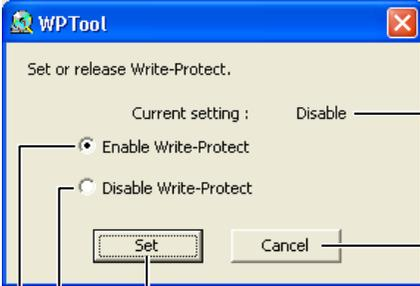
Displays the write-protect condition of the DVD-RAM disc currently loaded.
